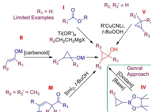
**Figure 1.** Cyclopropanols synthesis overview: (I) Kulinkovich reaction, (II) Simmons-Smith reaction, (III) visible-light-induced organocatalysis, (IV) oxidative hydrolysis of cyclopropylboronates, and (V) radical-mediated cyclopropanation.
