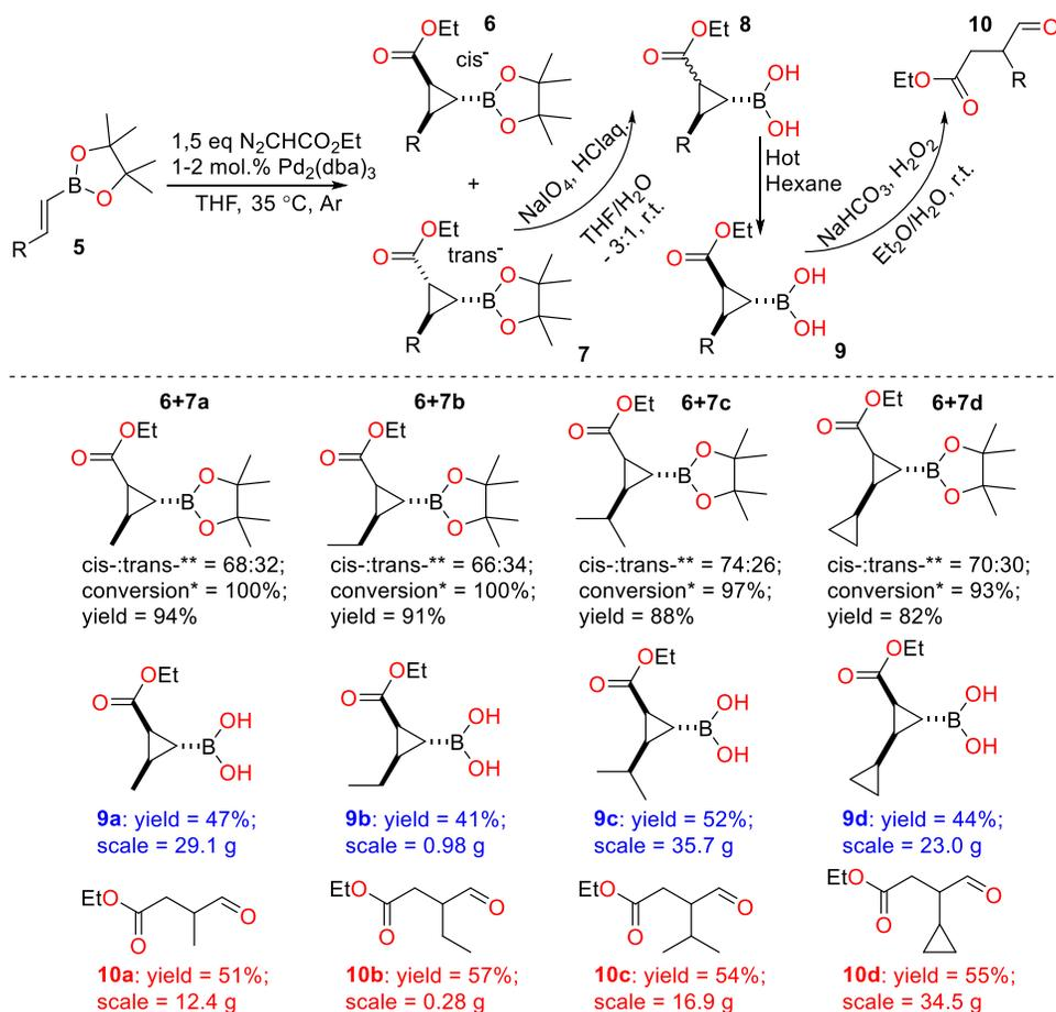
**Figure 4.** Preparation of *trans*-carbethoxy cyclopropylboronic esters (**6+7a-d**) and their sequential oxidative hydrolysis to cyclopropylboronic acids (**9a-d**) and ester-aldehydes (**10a-d**). \*Conversion was determined via  $^1\text{H}$  NMR analysis of the reaction mixture. \*\**cis*:*trans* ratio was determined by GC/MS analysis of purified products.
