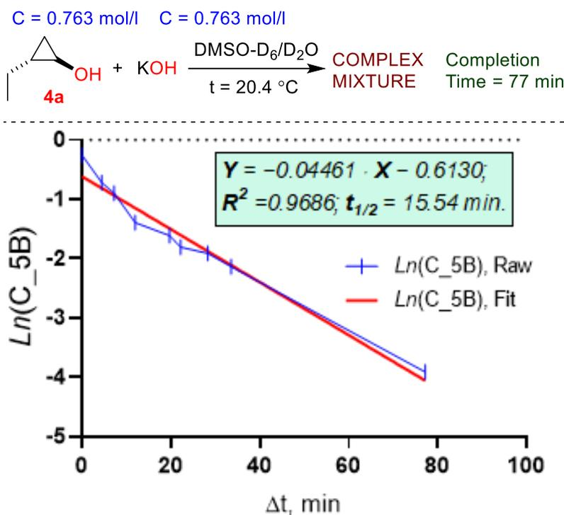
**Figure 3.** NMR-kinetic study of *trans*-2-ethylcyclopropan-1-ol (**4a**) decomposition in DMSO- $D_6/D_2O$  with KOH at room temperature.
