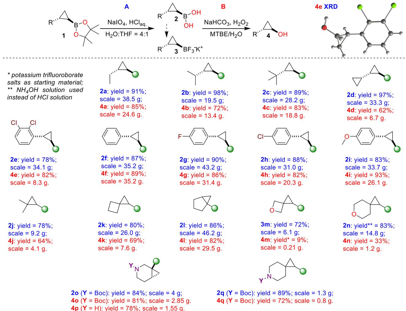
**Figure 2.** The two-step protocol for cyclopropanols (**4a-q**) and cyclopropylboronic acids (**2a-q**) synthesis via sequential oxidative hydrolysis of cyclopropylboronic esters (**1**).
