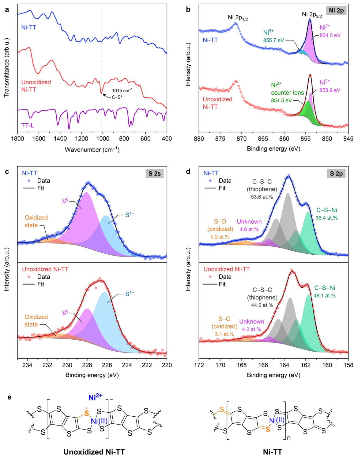
**Figure 3.** (a) Closed-up FTIR spectra showing the radical character. High-resolution XPS spectra of (b) Ni 2p, (c) S 2s, and (d) S 2p. (e) Proposed chemical structures of **Unoxidized Ni-TT** and **Ni-TT**.
