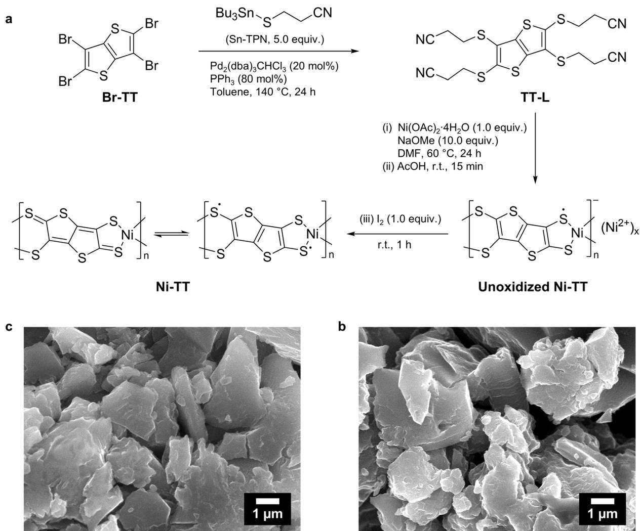
**Figure 1.** (a) Schematic synthesis and proposed chemical structures of **Unoxidized Ni-TT** and **Ni-TT**, along with their SEM images (b-c).
