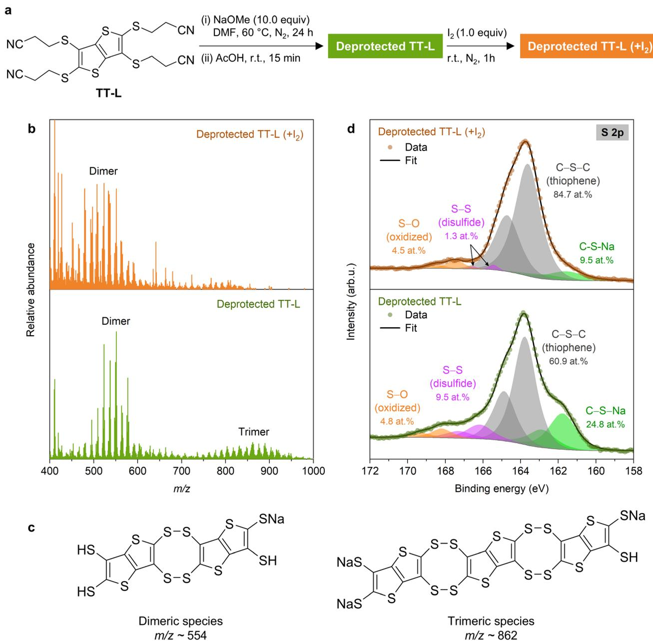
**Figure 4.** (a) Schematic synthesis of **Deprotected TT-L** with and without the addition of  $I_2$ . (b) Full scan APCI mass spectra. (c) Proposed chemical structures of the by-products. (d) High-resolution S 2p XPS spectra of the deprotected ligand samples.
