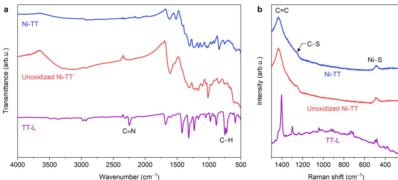
**Figure 1.** (a) FT-IR and (b) Raman spectra of **Unoxidized Ni-TT** and **Ni-TT**. Data of **TT-L** are also shown for reference.
