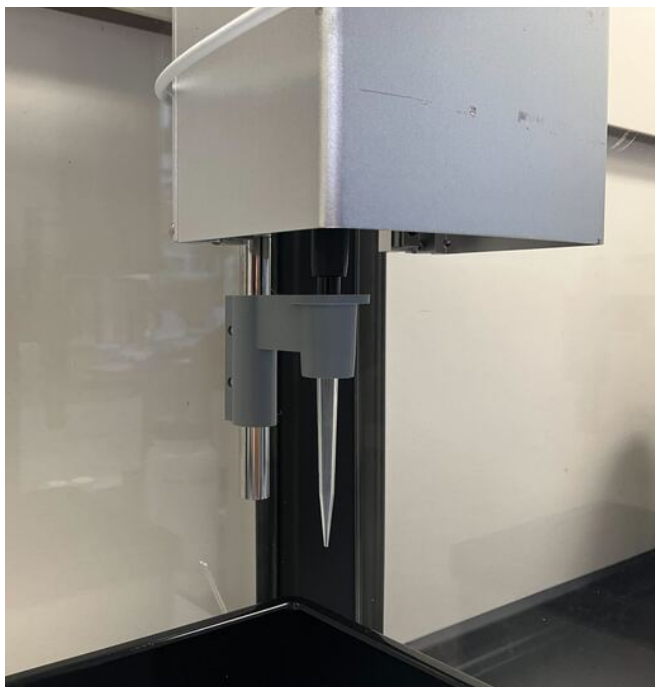
Figure 3. Close-up of the robotic pipetting gantry with a custom 3D-printed pick-and-place apparatus, holding a pipette tip and camera mount.
