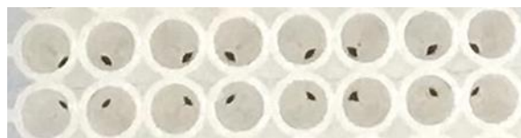
Figure 3: 96-well plate wells with magnetic beads attracted to SISCAPA magnet underneath
