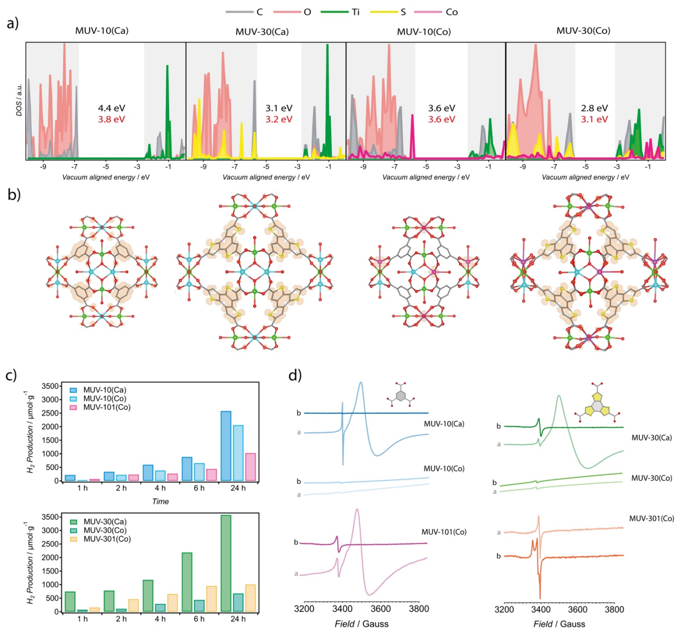
Figure 6. a) Electronic DOS spectra aligned relative to the vacuum level and b) electron density of the highest occupied crystalline orbital of MUV-10(Ca), MUV-30(Ca), MUV-10(Co) and MUV-30(Co). The grey background areas in each plot are the HOCO and LUCO, and the white area between them indicates the theoretical band gap (in black) compared to the experimental value (red) obtained from the Tauc plots. c) Cumulative H 2 photogeneration plots over time grouped by organic connector used in each family: BTC ( top ) and BTT ( bottom ). The activities of MUV-10 and 30 based on the Ti 2 Ca 2 cluster present activity maxima for each family. d) EPR spectra of all solids before (dark line) and after (light line) irradiation with a Kessil PR160L-370 nm. Ti 3+ formation corresponding to resonances with g-factors lower than 2.0 is observed only for MUV-10(Ca), MUV-30(Ca), and MUV-101(Co).
