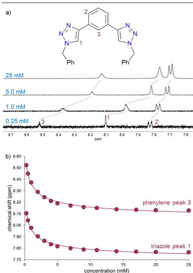
**Figure 2**  $^1\text{H}$  NMR study of self-aggregation of **2** in 9:1  $\text{CDCl}_3:\text{d}_6\text{-acetone}$  (298 K): a) partial  $^1\text{H}$  NMR spectra of **2** at various concentrations; b) chemical shift of interior phenylene and triazole C–H resonances at various concentrations (circles represent data, lines represent dimerization isotherm calculated using *Bindfit*<sup>37</sup>).
