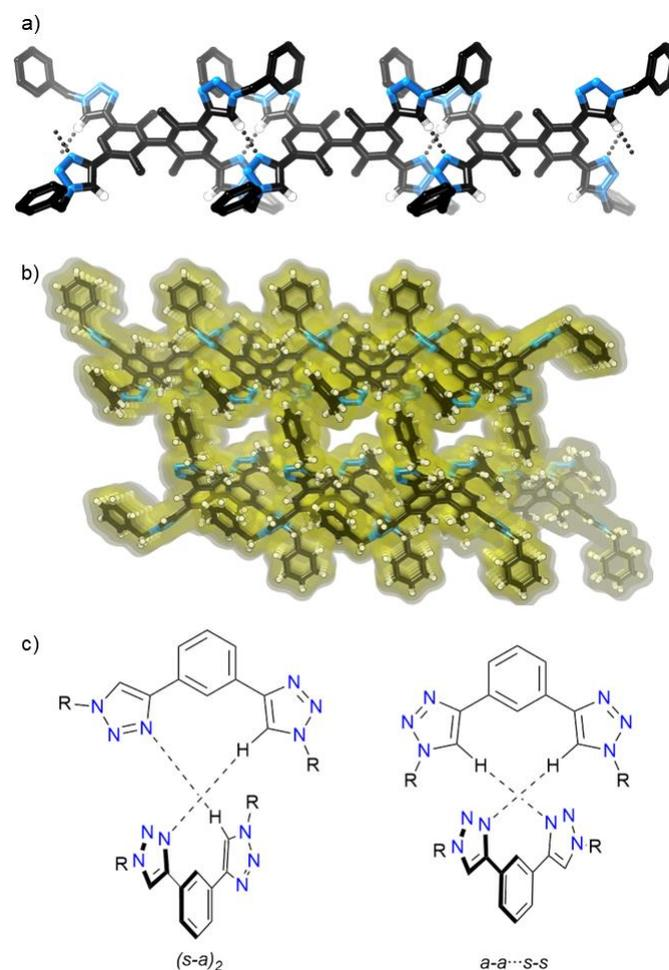
**Figure 3** X-ray crystal structure of **1<sub>DCM/pentane</sub>**: a) 1D hydrogen-bonded chain, b) packing diagram showing small 1D channels, c) two possible hydrogen bonding arrangements between phenyl-1,3-bis(triazole) groups. Most hydrogen atoms are omitted in part a), in part b) the van der Waals' radii of the atoms are shown in yellow showing the small channels running through the structure. Solvent molecules are omitted in both parts.
