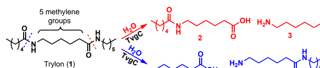
Scheme 1. The two amides in 1 are not equivalent and can be hydrolyzed to release two different sets of products
