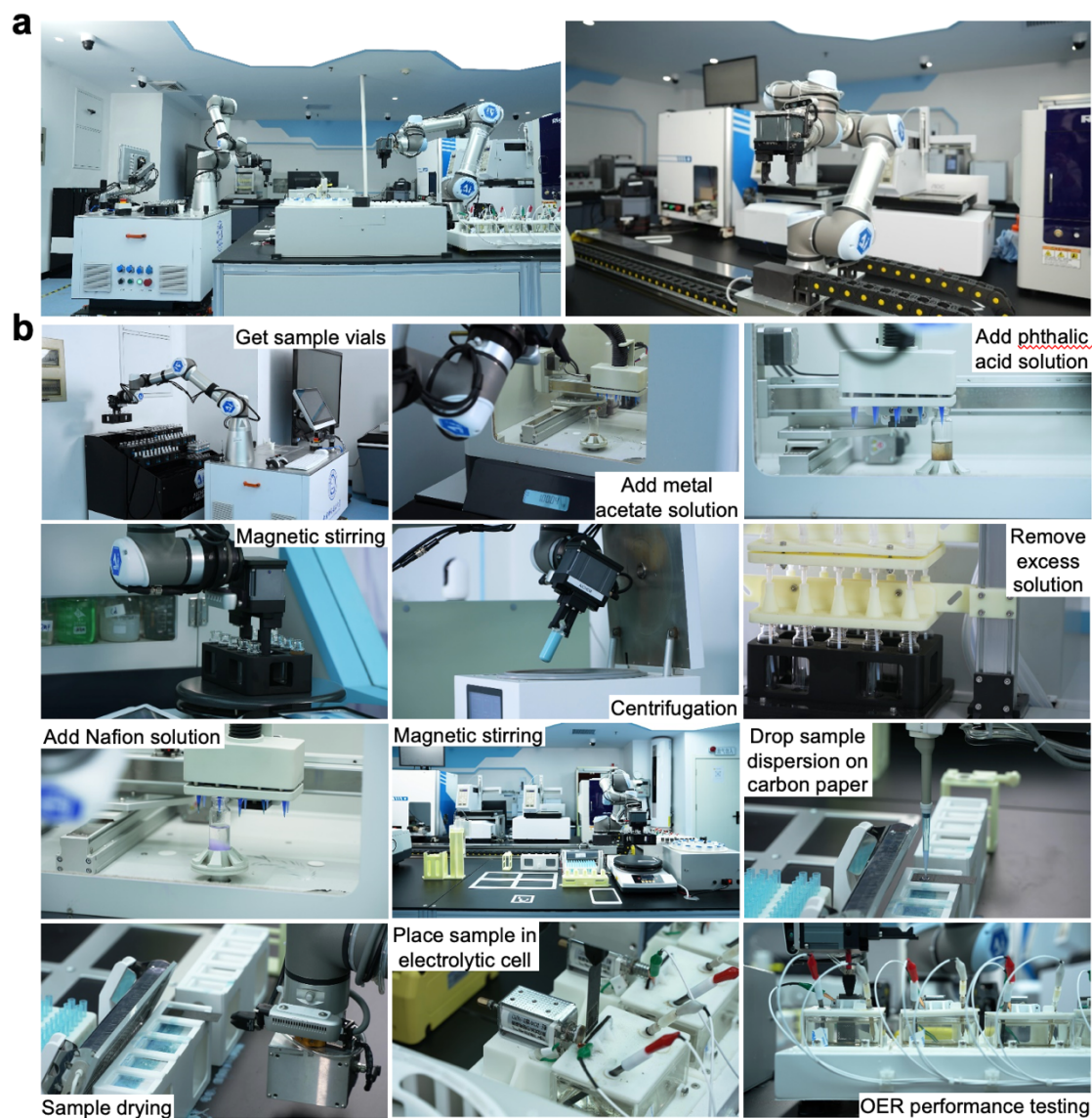
Extended Data Figure 1: The Automated Lab. a , Depiction of the two experiment-conducting robots: a fully mobile robot and a benchtop robotic arm. b , Examples of key robotic operations along the autonomous workflow for sample synthesis and electrochemical testing.
