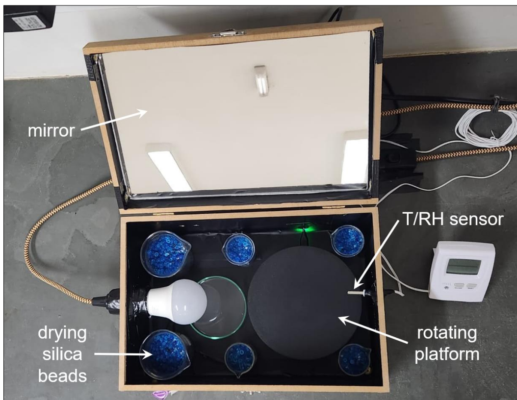
Figure S1 - Home-made setup used for the light-accelerated degradation test. The samples were distributed uniformly in the Petri dish, which was positioned in the center of the rotating (6 Hz clockwise) platform and submitted to direct and mirror-reflected illumination from the LED lamp. The lamp specifications are a power of 6 W, luminous flux of 560 lm, and color cold white (6500 K). The box (30 x 20 x 15 cm) remained closed and sealed with masking tape during the test. Inside humidity was kept as low as possible by drying silica beads. Temperature and relative humidity were constantly monitored.
