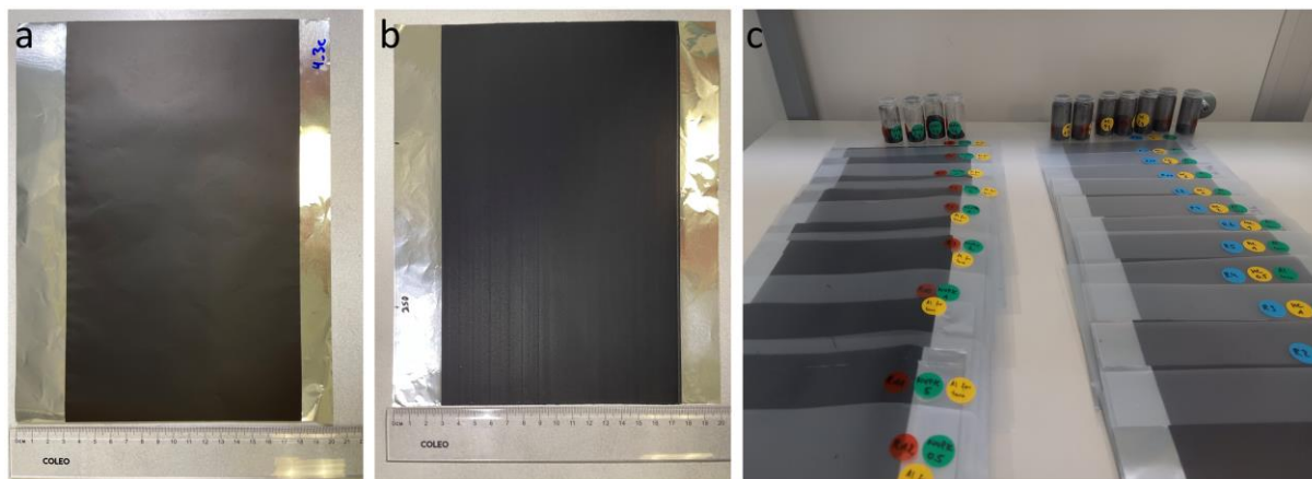
Figure 5. Photos of a) a sheet of the hard carbon reference anode, b) a sheet of the NVP/C reference cathode and c) the preparation for the distribution of active material powders and electrodes for further studies.
