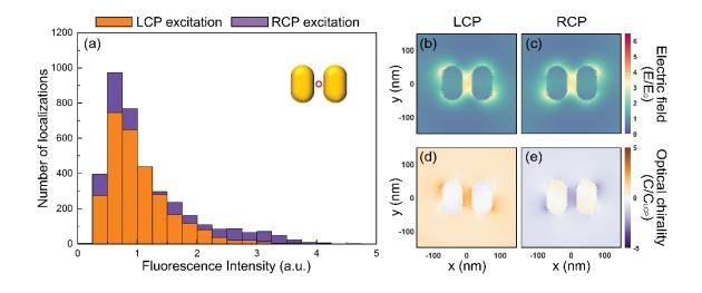
Figure 2. Experimental and computational optical characteristics around achiral Au NP dimer antennas under left and right circularly polarized light (LCP and RCP, respectively).
