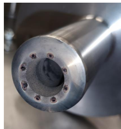
Figure 2: Accumulation of powder on burner orifices was observed
