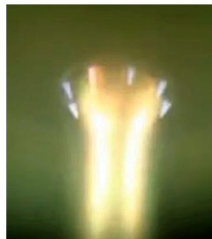
Figure 4: Flame emission when Cu-powder is fed into the flame
