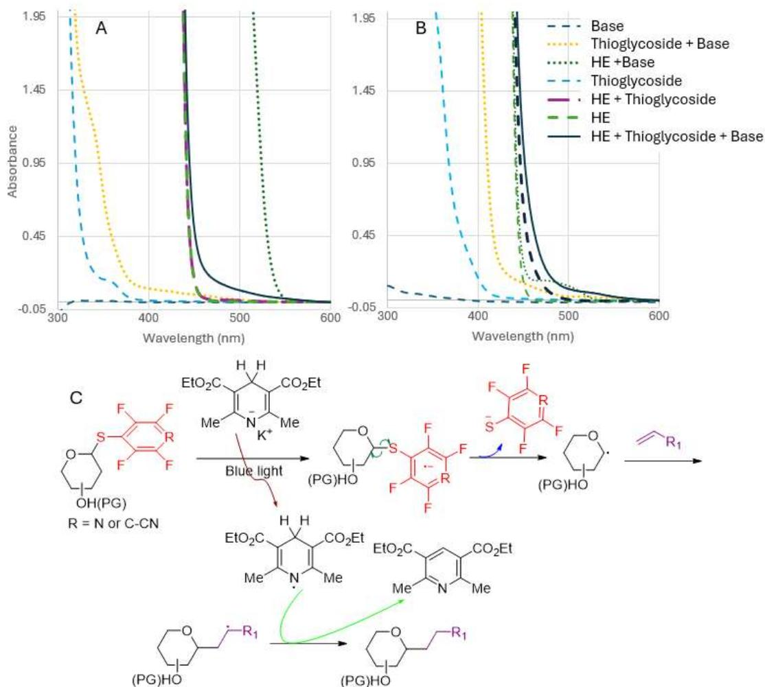
Figure 3. Absorbance spectra and proposed mechanism of photoinduced desulfurative radical coupling. A. Thioglycoside **12**, Base  $K_2CO_3$ , B. Thioglycoside **13**, Base  $KHCO_3$ . C. Proposed mechanism
