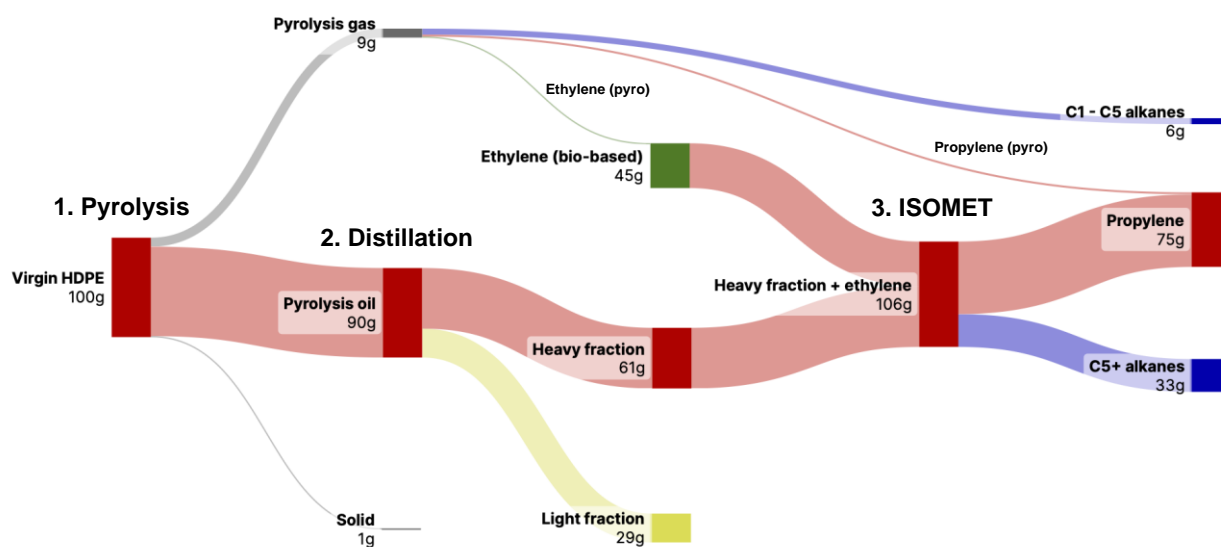
Figure 6. A Sankey diagram representing the total mass balances of the HDPE polymer pretreatment and ISOMET process. The complete olefin ISOMET conversion of the heavy fraction was demonstrated on municipal HDPE plastic waste pyrolysis oil. The remaining alkanes can be further utilized by pyrolysis or catalytic dehydrogenation.
