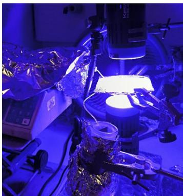
Figure S2. Gram scale synthesis reaction setup of 2a.
