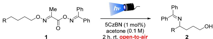
To an 8 mL vial equipped with a magnetic stir bar was added the bifunctional reagent **1** (0.25 mmol, 1.0 equiv), 5BzCN (2 mg, 2.30  $\mu\text{mol}$ , 1 mol%) and acetone (2.5 mL, c = 0.1 M). The vial was sealed with a cap containing a Sil/PTFE septum, and the reaction mixture was irradiated with a Kessil PR160-blue LED lamp (30 W High
