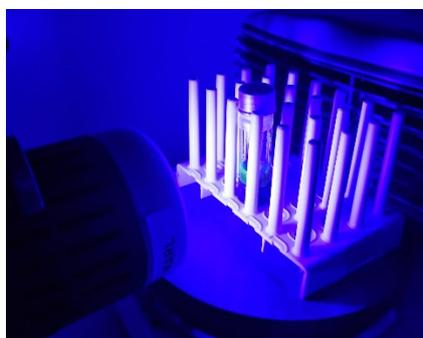
**Figure S1.** Reaction setup for the visible light-assisted synthesis of 1,5-aminoalcohols and 1,5-diamines
