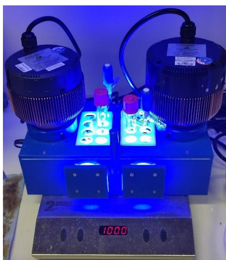
Figure S1. Hepatochem EvoluChem™ PhotoRedOx Box Duo with irradiation by EvoluChem™ HCK1012-01-008 blue LEDs (30 W, \lambda_{\text{max}} = 450 nm).
