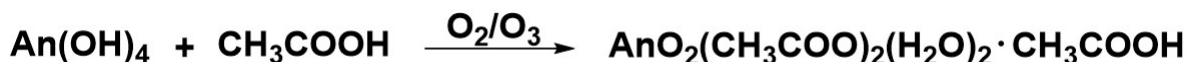
Figure 2: Synthetic scheme for accessing AnO 2 (CH 3 COO) 2 (H 2 O) 2 ·CH 3 COOH (An = U, Np, and Pu) by direct oxidation with oxygen or ozone.
