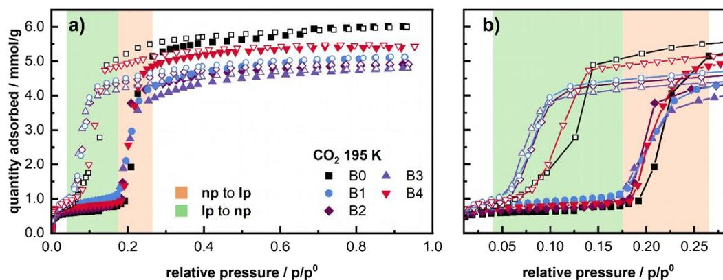
**Figure 4.** a) CO<sub>2</sub> physisorption isotherms of **B0-4**. Steps in the isotherms correspond to framework opening during adsorption (**np** to **lp**, light orange) and closing during desorption (**lp** to **np**, green). b) Highlighted pressure range of the low-pressure region, where the phase transitions occurs. Adsorption and desorption depicted in full and open symbols, respectively; lines have been added as visual aid only.
