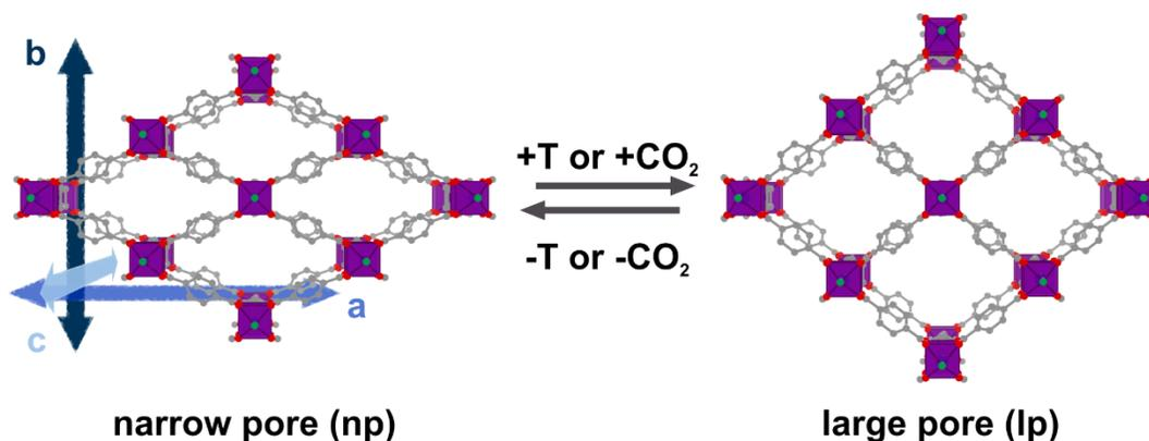
**Figure 1.** Visualization of  $\text{Zn}_2(\text{BME-bdc})_2\text{dabco}$  and directions of unit cell parameters a, b, and c. The MOF exhibits a switchable phase transition from its narrow pore (**np**) phase lozenge-lattice to its large pore (**lp**) phase square-lattice. View along the stacked dabco pillars in c direction. C, grey; O, red; N, green; Zn coordination polyhedron, purple; hydrogen atoms and BME functionalization of the bdc linker is not shown for clarity.
