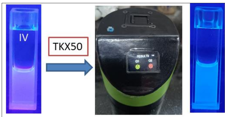
Fig. 8 Working procedure of the developed prototype for detection of TKX 50 via visual response.
