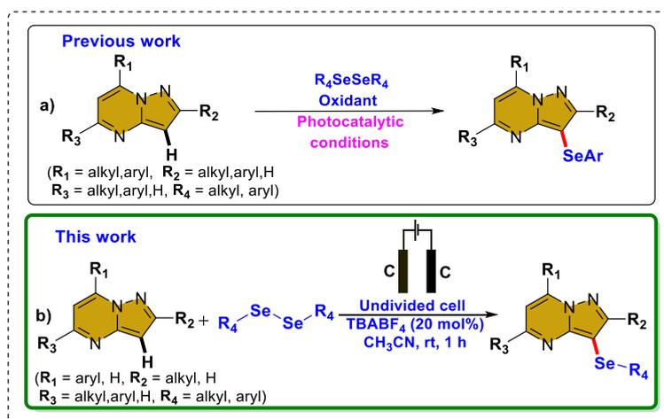
**Scheme 1.** Previous work on selenylation of pyrazolo[1,5-*a*]pyrimidines
