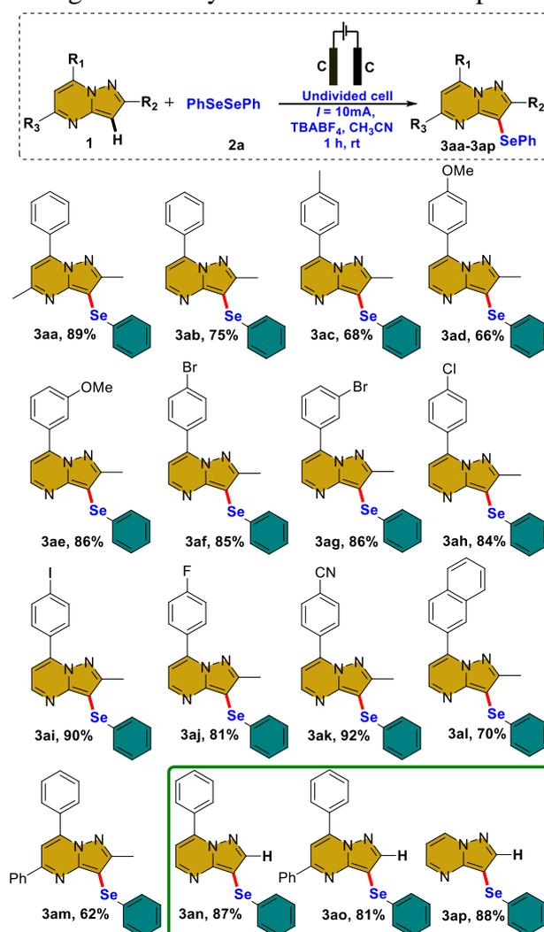
**Scheme 2.** Substrate scope for electrochemical selenylation of pyrazolo[1,5-*a*]pyrimidines. <sup>[a]</sup>Reaction conditions: **1** (0.2 mmol), **2a** (0.1 mmol), TBABF<sub>4</sub> (20 mol%), CH<sub>3</sub>CN 4.0 mL, constant current ( $I = 10$  mA), rt, reaction mixture was electrolysed in Electrasyn 2.0 instrument for 1 h. Yields are isolated yields.
