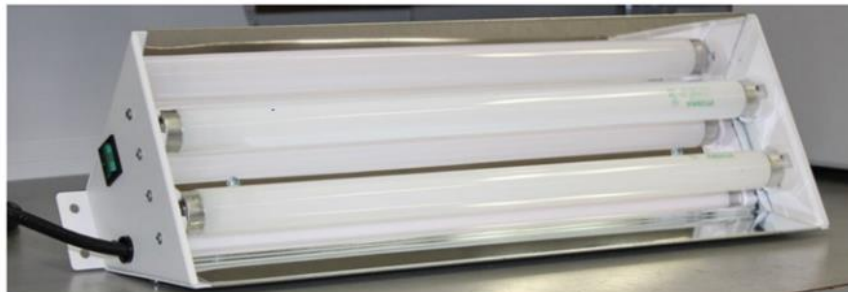
Figure 4. Visualisation of the XX-15 UV device with monochromatic 254 nm lamps.
