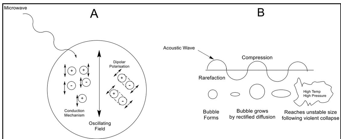
**Figure 4:** (A) Microwave effects on the polarizability of polar solvents, as well as local heating or superheating causing increased reaction rates. (B) Acoustic waves (sonicator) causing compression and rarefaction causing increased mechanical effects causing increased reaction kinetics.
