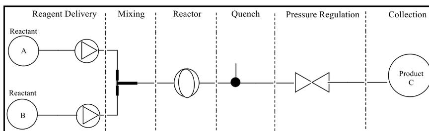
**Figure 1:** Six component breakdown of a basic flow system with coil reactor
