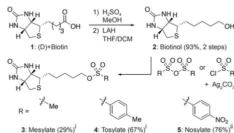
**Scheme 1.** Synthesis of a panel of electrophilic biotin initiators. Mesylate **3**, tosylate **4**, and nosylate **5** were all accessed from a common biotinol precursor. i) Sulfonate anhydride, pyridine, DCM, rt. ii) 4-nitrobenzene sulfonyl chloride, pyridine, Ag<sub>2</sub>CO<sub>3</sub>, DCM, rt.
