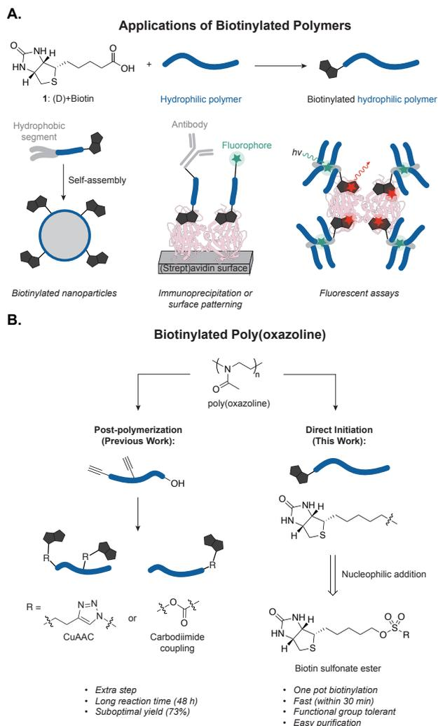
**Figure 1.** Biotinylation of hydrophilic polymers. A) Applications of biotin polymers. B) Previous work on biotinylated P(Ox) relies solely on post polymerization modifications. Work described herein: rapid and direct biotinylation of P(Ox) using an electrophilic initiator.
