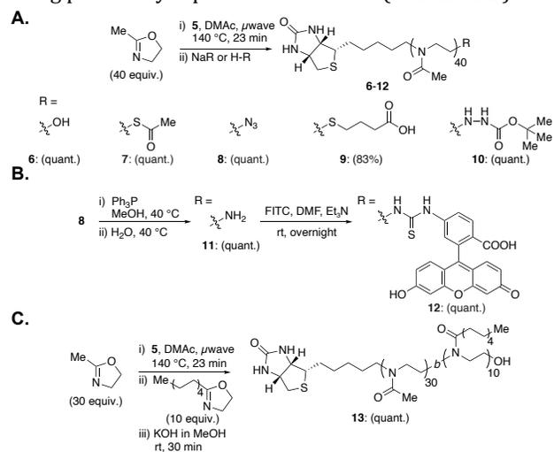
**Scheme 2.** End group panel of biotin-P(MeOx). A) Terminal functionalization with strong nucleophiles. B) Post polymerization modification of biotin-P(MeOx). C) Synthesis of biotinylated diblock co-polymer P(Ox) surfactant.
