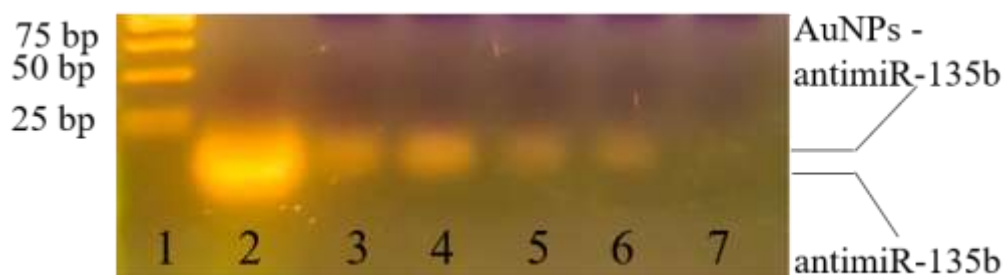
Figure 6. Confirmation of the antimir-135b - AuNPs conjugation. Different concentrations of antimir-135b are shown. 1) MassRuler low range DNA ladder, 2) control antimir-135b (100 mM), 3) AuNPs-50 mM of antimir-135b, 4) AuNPs-40 mM of antimir-135b, 5) AuNPs-30 mM of antimir-135b, 6) AuNPs-20 mM of antimir-135b, 7) FP.
