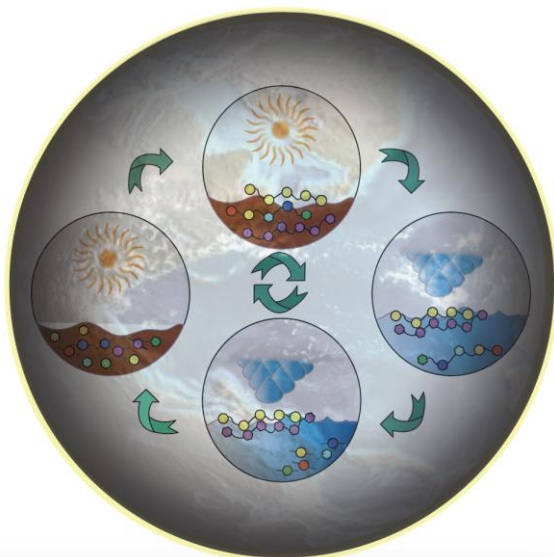
Fig. 1. Wet-dry cycling. During dry conditions, molecules condense to form larger, more complex molecules. During wet conditions, complex molecules are partially hydrolyzed back to smaller, simpler molecules. Experimental wet-dry cycling mimics conditions on land surfaces of the earth.
