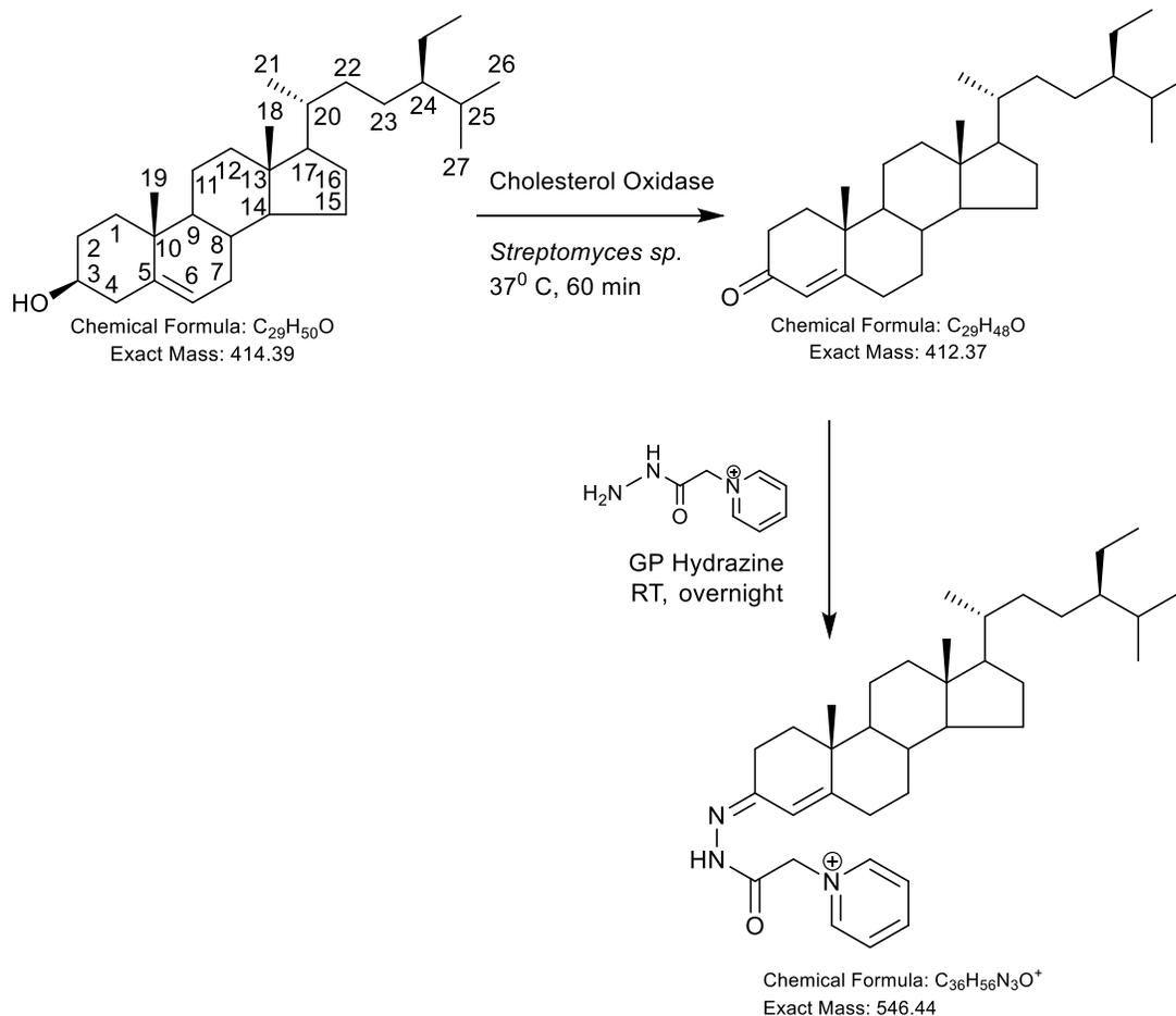
**Figure 2.** Enzyme-assisted derivatization for sterol analysis EASDA. Example is shown for  $\beta$ -sitosterol, of which 3 $\beta$ -hydroxy group was converted to 3-oxo group followed by GP reagent derivatization to GP hydrazone, O/GP  $\beta$ -sitosterol.
