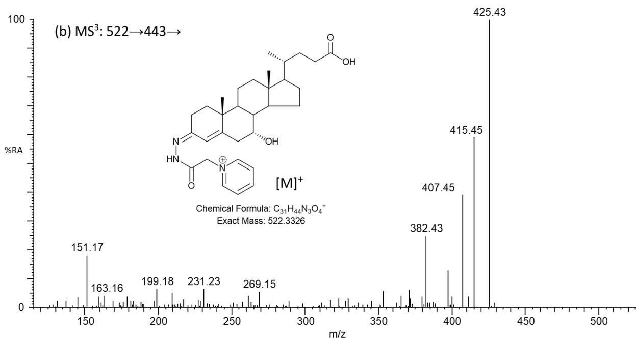
**Figure 12.** (a) LC-MS RICs of MS<sup>3</sup> (522 → 443 →) transition, (b) MS<sup>3</sup> spectrum recorded at 2.01 min corresponding to the O/GP derivatized 7 $\alpha$ -hydroxy-3-oxocholest-4-enoic acid.
