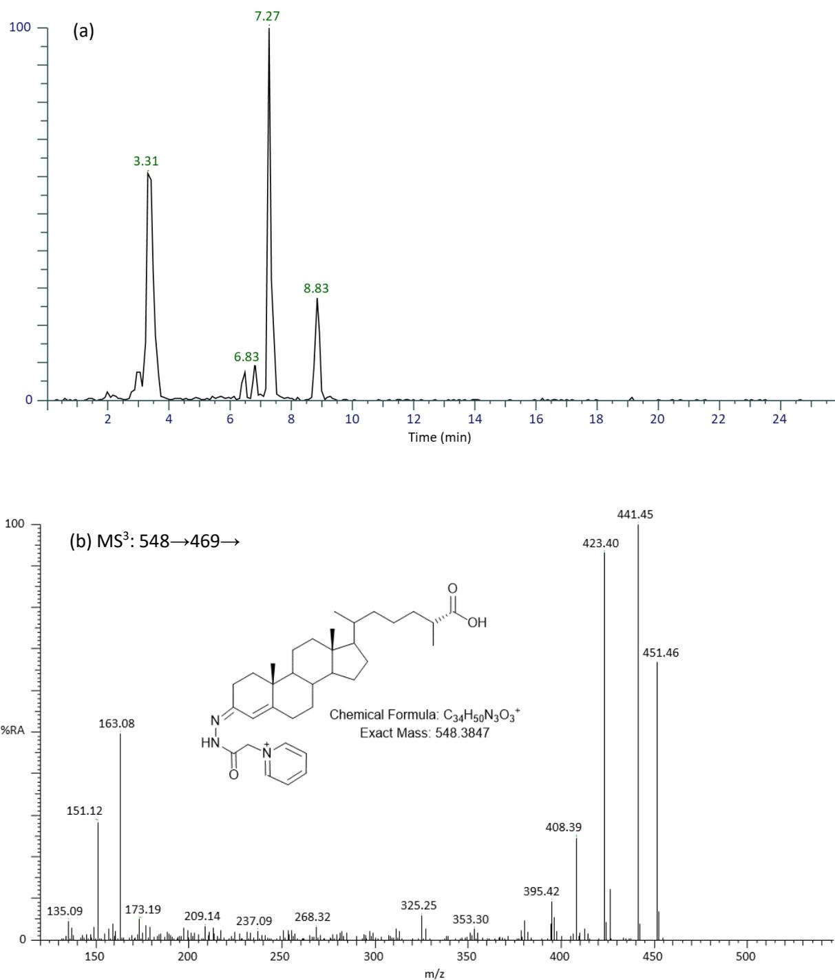
**Figure 11.** (a) LC-MS RICs of MS<sup>3</sup> (548→469→) transition corresponding to O/GP-sterols formed after EADSA protocol application using serum sample from an AHC patient. The MS<sup>3</sup> (548→469→) spectrum of component eluting at (b) 3.31 min corresponding to 3β-hydroxycholest-(25R)-5-en-26-oic acid.
