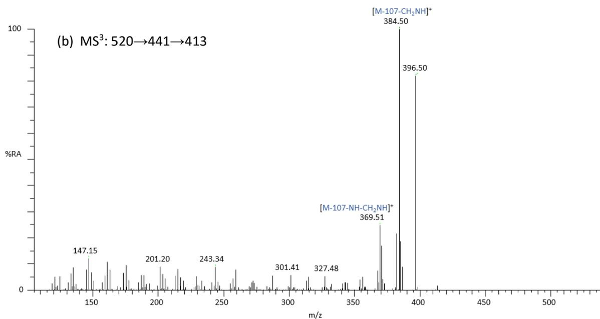
**Figure 7.** (a) The MS<sup>3</sup> (520.5→441.5→) spectrum, and (b) MS<sup>4</sup> (520.5→441.5→413.5→) spectrum of O/GP-derivatized cholesterol authentic standard.
