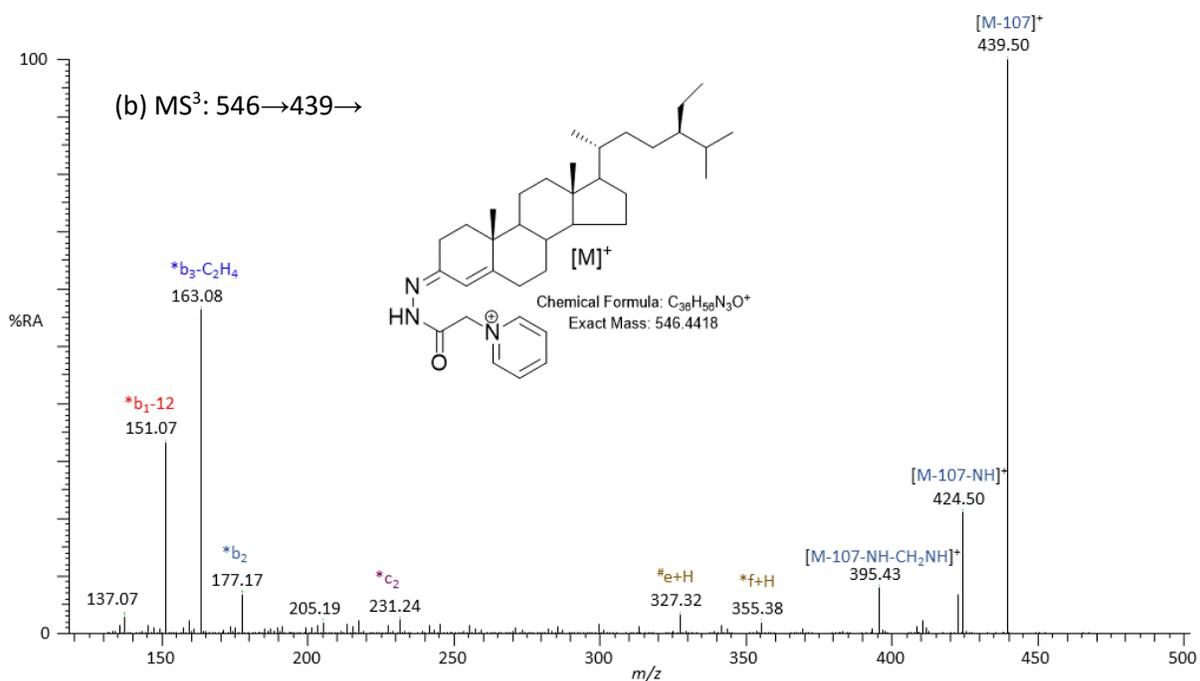
**Figure 3.** (a) ES-MS<sup>2</sup> (546→); and (b) MS<sup>3</sup> (546→439→) spectra of the oxidized and GP-derivatized  $\beta$ -sitosterol authentic standard.
