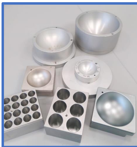
Figure 20: Metal heating block as efficient and safe replacement for oil heating baths.
