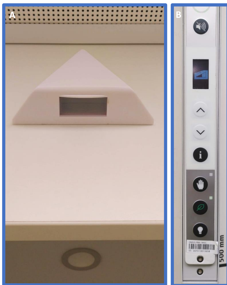
Figure 15: a) Ensure that the light sensors are functional at all times. b) Do not change the settings of the fume hood to keep the automated closing system enabled.
