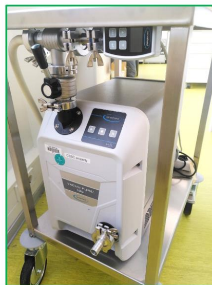
Figure 21: Screw pumps as replacement for oil pumps. For cold traps utilize frozen isopropanol instead of liquid nitrogen or frozen acetone. It is the preferable choice with a melting point of -89^{\circ}\text{C} , sufficient in almost all cases, and has better freezing and environmental properties.
