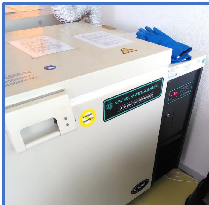
Figure 17: Increase the temperature of a -80^{\circ}\text{C} freezer to -70^{\circ}\text{C} to save energy. An ultra-low temperature freezer consumes as much energy as a household annually. 56
