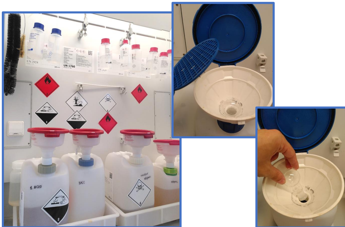
Figure 3: Funnels with lid to prevent solvent evaporation from waste canisters (left). Use of a round bottom flask to improve solvent loss by evaporation, which can serve as alternative to funnels with a lid (right). Another alternative to the round bottom flask is the plastic balls used to cover water baths in rotary evaporators (see Section 4 ), which can also be placed in a funnel to prohibit solvent loss by evaporation.
