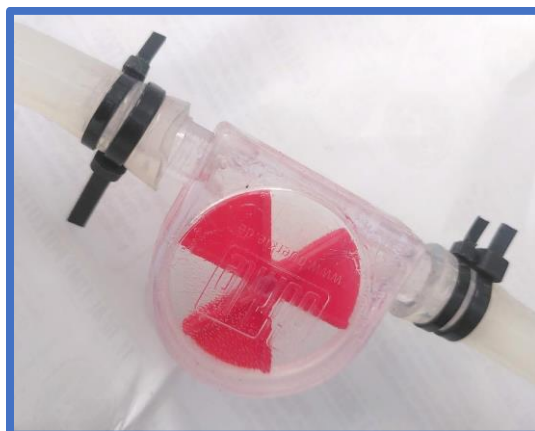
Figure 13: Paddle wheel flow meters or water wheels to monitor flow of cooling liquid.
