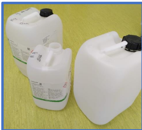
Figure 4: Reuse of solvent bottle (e.g. ethanol or acetone) and repurposing it as waste canister to avoid ordering new waste canisters for disposal. For safety, one needs to remove the previous label and stickers and add the respective waste label.
