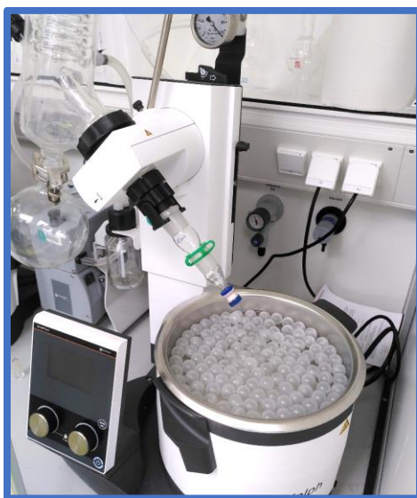
Figure 19: Plastic balls in the water bath of a rotary evaporator to prevent energy loss in form of heat.
