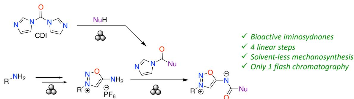
The mechanochemical synthesis of N6-functionalized iminosydnone salts was performed via a convergent strategy based on the desymmetrization of CDI. The whole process was carried out by ball-milling, offering an efficient and sustainable access to bioactive iminosydnone salts.
