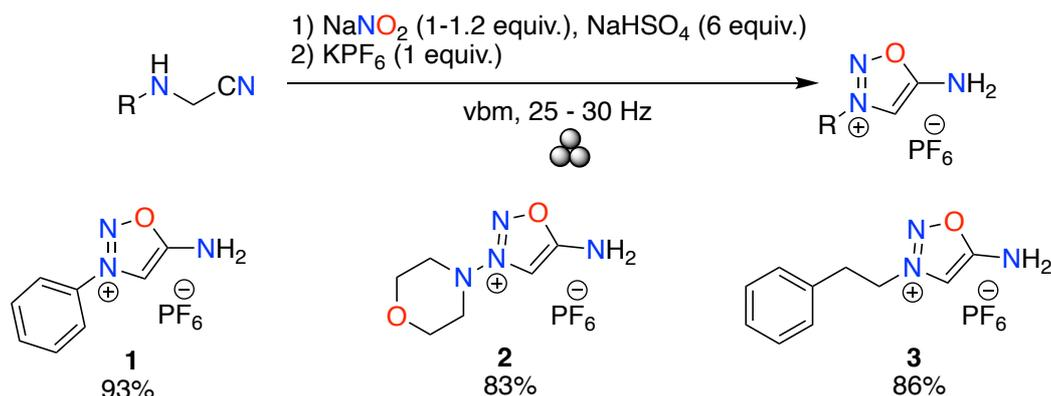
**Scheme 2. Mechanochemical synthesis of the iminosydnone core**
