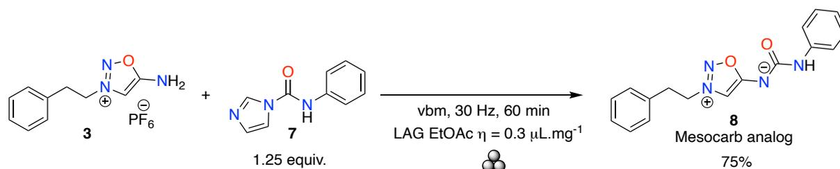
**Scheme 5. Mechanochemical Mesocarb analog synthesis**
