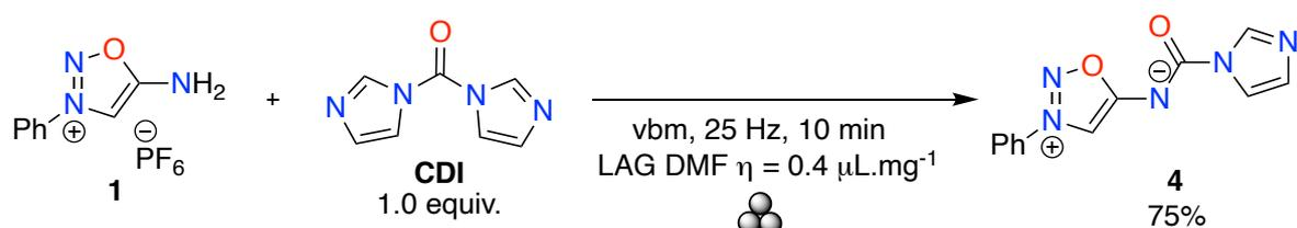
**Scheme 3. Mechanochemical synthesis of ImSyd-carbonylimidazole intermediate**
