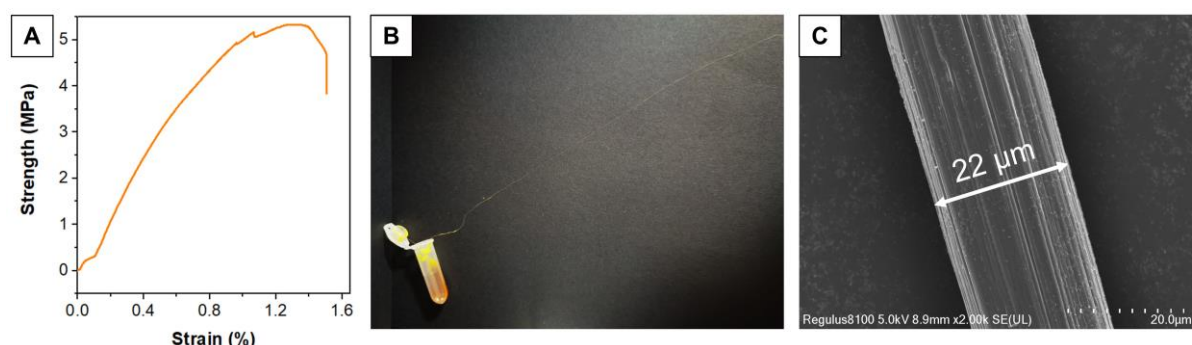
Figure S13. Mechanical properties of P1a2aCS 2 . (A) The stretch curve of P1a2aCS 2 tested by electronic universal testing machine. (B) The continuous fiber of P1a2aCS 2 prepared through solution processing and (C) the scanning electron microscope image of this fiber.
