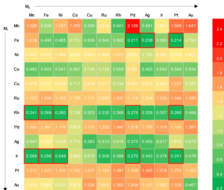
Figure 2. Overpotential of the 144 SACs. Green values indicate low overpotential (high activity), Orange/Red values indicate high overpotential (low activity). Promising SACs with \eta < 0.304 V are highlighted with red squares.
