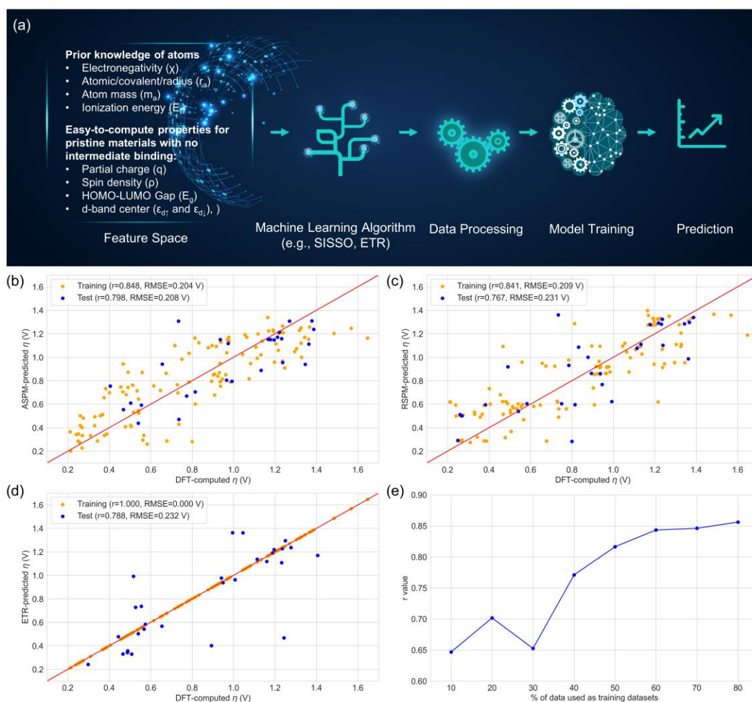
Figure 6. (a) Workflow of the ML process for predicting overpotential from intrinsic atomic properties and DFT-computed electronic properties. Prediction performance of the (b) ASPM SISSO, (c) RSPM SISSO, and (d) ETR models for the training (80%) and testing (20%) datasets. (e) Illustration of the incremental improvement in the predictive ability of the ETR model with increasing size of training datasets.
