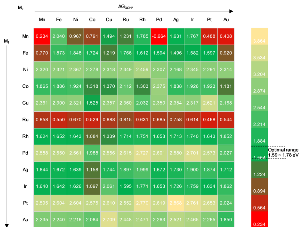
Figure 4. \Delta G_{\text{OOH}}^* for 144 SACs. Optimal binding energies ( \sim 1.59 – 1.78 eV) are represented in green, overly strong binding energies are marked in red, and excessively weak binding energies are denoted in yellow.
