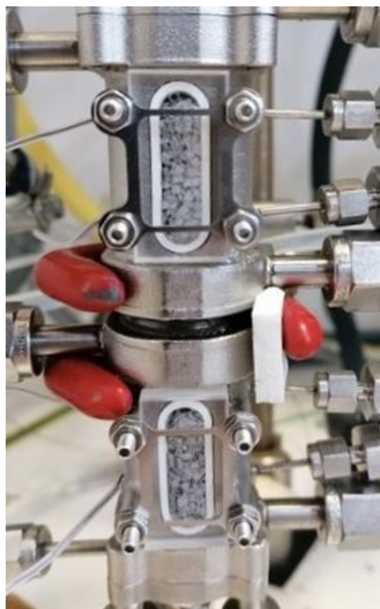
Figure 12: Precipitation during continuous lab scale synthesis of pentylmagnesium iodide in THF. Magnesium turnings are covered with white precipitate.
