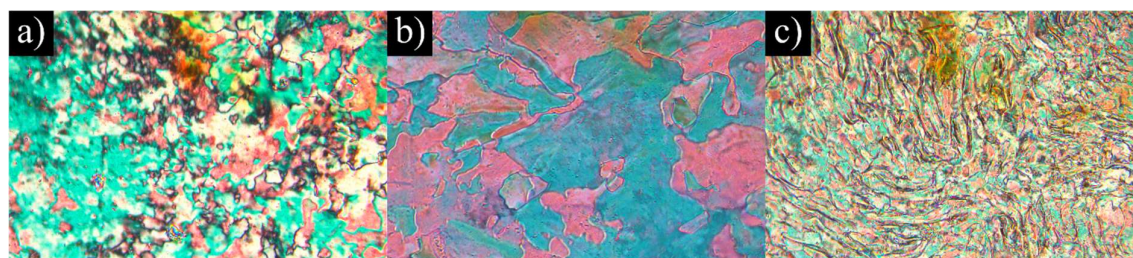
Figure 3. POM textures of 3JK. a) Marble-like texture of N phase (T=115°C), b) N F texture in the heating cycle (T=85°C), c) N F texture in the cooling cycle (T=85°C).
