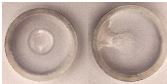
FIG 4: Reaction of titanium(IV) propoxide liquid with moisture from the air. On the left titanium(IV) propoxide under dry air conditions, on the right a droplet of titanium(IV) propoxide exposed to natural air after 5 minutes. Note the humid air exposed sample has turned to a chalky white, indicating the formation of TiO 2 and loss of original liquid structure.
