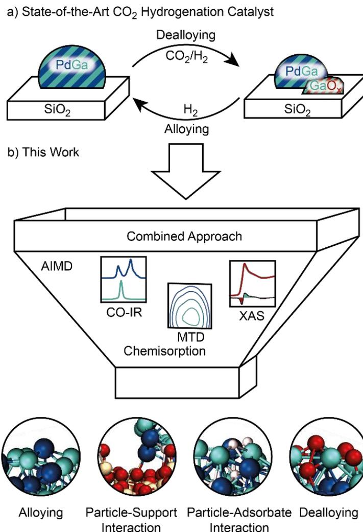
**Fig. 1:** a) State-of-the-art CO<sub>2</sub> hydrogenation catalyst based on a PdGa alloy supported on a dehydroxylated silica support and its complex alloying-dealloying behavior under reaction conditions. b) Combined computational and experimental approach of this work to elucidate the atomic level structure of (de)alloying, particle-support, as well as particle-adsorbate interactions.
