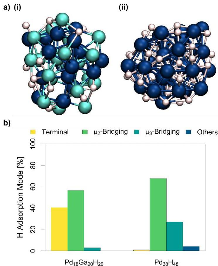
**Fig. 4.** a): Structure of (i) Pd<sub>18</sub>Ga<sub>20</sub>H<sub>20</sub> NP and (ii) Pd<sub>38</sub>H<sub>48</sub> NP in vacuum obtained from Metadynamics. Pd: dark blue, Ga: brighter blue, and H: white (trajectories and FES can be found in Fig. S47-S68). b): Proportion of different hydride coordination modes of the Pd<sub>18</sub>Ga<sub>20</sub>H<sub>20</sub> and Pd<sub>38</sub>H<sub>48</sub> NP obtained from AIMD simulations.
