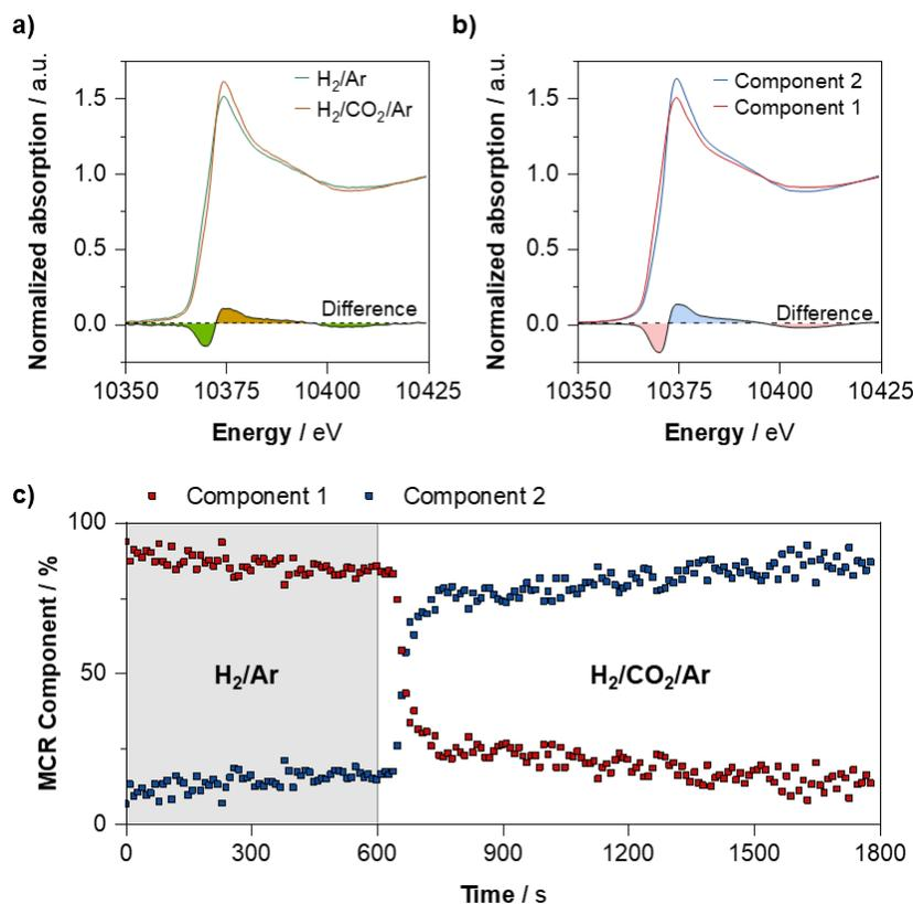
**Fig. 5:** Ga K edge XANES of PdGa@SiO<sub>2</sub> under reaction conditions. a) before and after introduction of CO<sub>2</sub>, b) pure spectral components obtained from a 2-component MCR fit tracking introduction of CO<sub>2</sub> into the gas phase, and c) MCR component profiles tracking influence of introduction of CO<sub>2</sub> to the reactive gas mixture.
