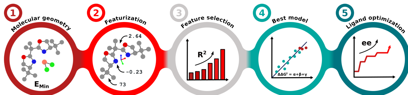
Figure 2: General workflow for model selection. (1) Ligands are optimized with a metal center to obtain the desired geometry. (2) 232 features are extracted from the metal-free structure. (3) The most promising feature combinations are identified through testing. (4) The best features undergo cross-validation and the best Bayesian ridge regression (BRR) model is obtained. (5) This resulting model is used for ligand screening with BO.
