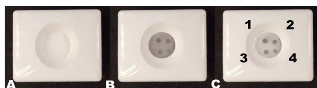
Fig. 2. Vertical flow assay procedure. A) Addition of analyzed sample; B) Addition of CNP@ MAb; C) Addition of 200 µl washing buffer. Spike-protein concentration: 1) 0.5 mg/mL; 2) 0.25 mg/mL; 3) 0.125 mg/mL; 4) 0.0625 mg/mL.
