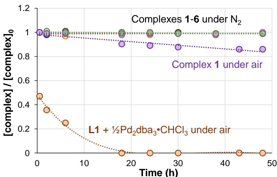
**Figure 4.** Concentration versus time plot for complexes **1-6** in THF under  $\text{N}_2$ , showing no decomposition over at least 48 h, as well as complex **1** and  $\text{L1} + \text{Pd}_2(\text{dba})_3 \cdot \text{CHCl}_3$  under air. These latter experiments show slow decomposition of **1** (>80% intact after 48 h) and rapid decomposition of  $[\text{L1}]\text{Pd}(\text{dba})$  (<50% remaining after 30 min).
