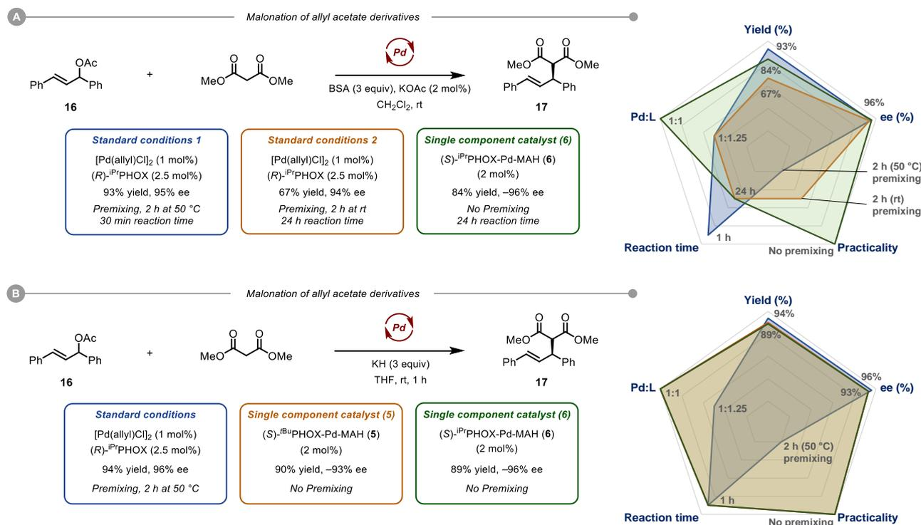
**Figure 6.** Comparison of established PHOX-type catalyst systems with new single-component precatalysts for benchmark AAA reactions. **(A)** Malonation of allyl acetate derivatives using weakly basic conditions for soft enolization. **(B)** Malonation of allyl acetate derivatives using strongly basic conditions to generate a potassium enolate nucleophile.
