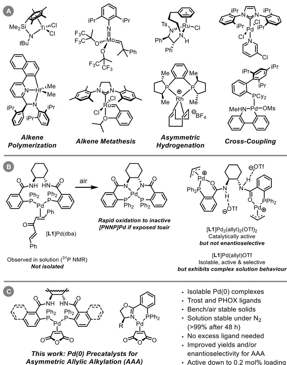
**Figure 1.** (A) Exemplar homogeneous organometallic precatalysts for specific transformations. (B) Challenges with accessing precatalysts containing Trost-type ligands, including rapid oxidation of Pd(0) species derived from Pd<sub>2</sub>(dba)<sub>3</sub>, and complex solution behaviour of Pd(II) allyl species. (C) This work: new single-component Pd(0) precatalysts for asymmetric allylic alkylation.
