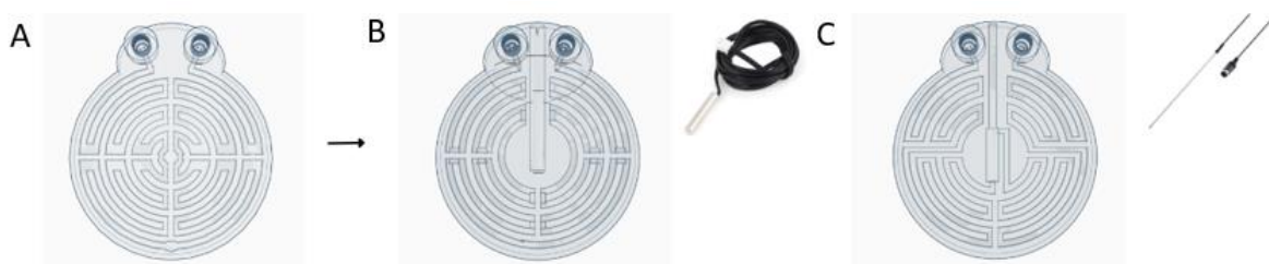
Figure 5: Tinkercad design illustrating reactor. A) First design of the Hilton Group. B) Modified reactor with the sensor cavity in the centre to incorporate a Digital Thermal Temperature Sensor. C) Modified reactor with the probe cavity in contact with the flow path.
