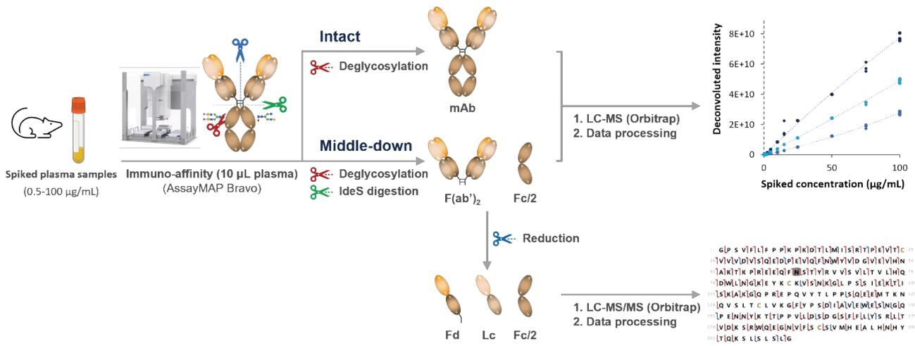
Figure 1: Overview of the developed automated workflow on the AssayMAP Bravo system combining immunocapture, top-down and middle-down LC-MS.
