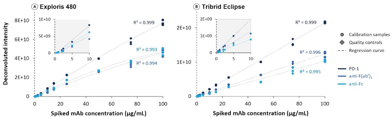
Figure 3: Calibration curves on the Orbitrap Exploris 480 (A) and Tribid Eclipse (B) for the total intact mAb semi-quantitation after immunocapture by PD-1 (dark blue), anti-F(ab')<sub>2</sub> (blue) and anti-Fc (light blue) antigens.
