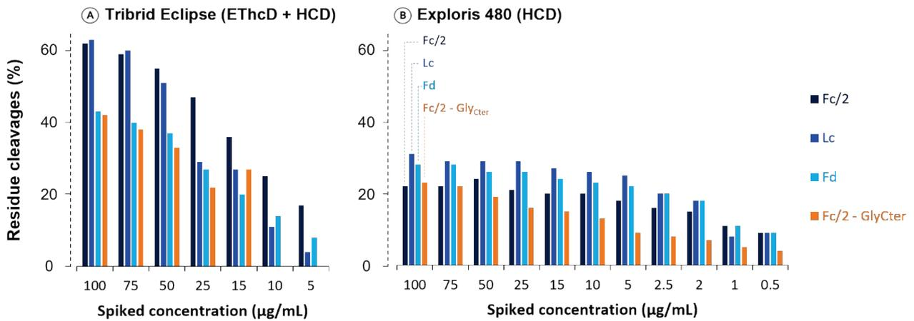
Figure 5: Sequence coverage in middle-down LC-MS/MS experiments for the four targeted mAb subunits on the Orbitrap Tribrid Eclipse (A) and Exploris 480 (B).
