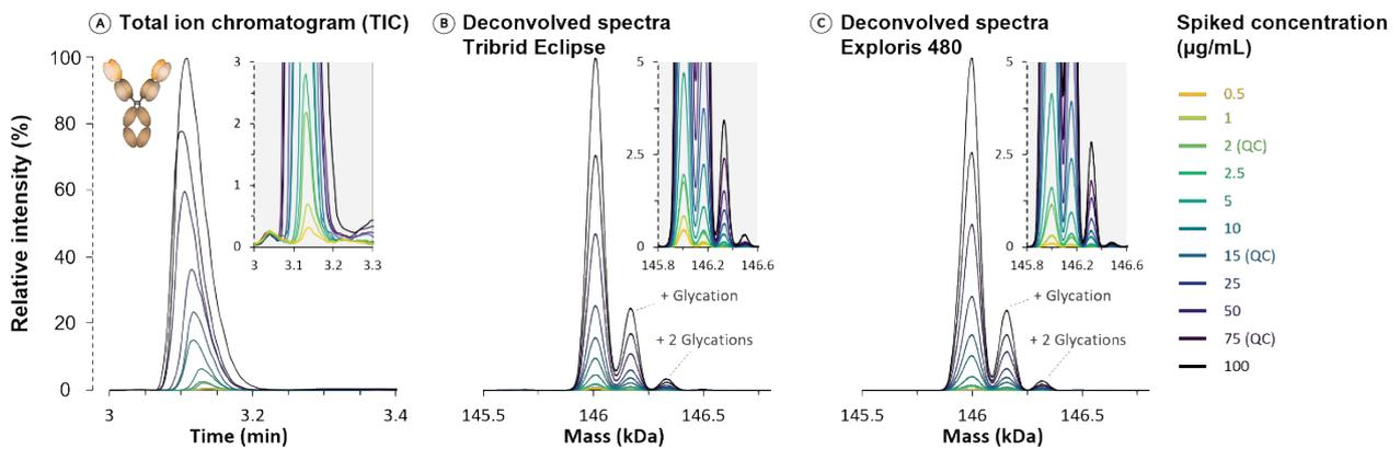
Figure 2: Total ion chromatogram (A) and deconvolved spectra (B – C) of intact pembrolizumab immunocaptured by PD-1 from mouse plasma (0.5 – 100 µg/mL) and deglycosylated. QC: quality control.
