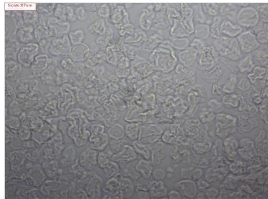
**Figure 20** - Microscopy of the starch solution after heating used in the MF process.
