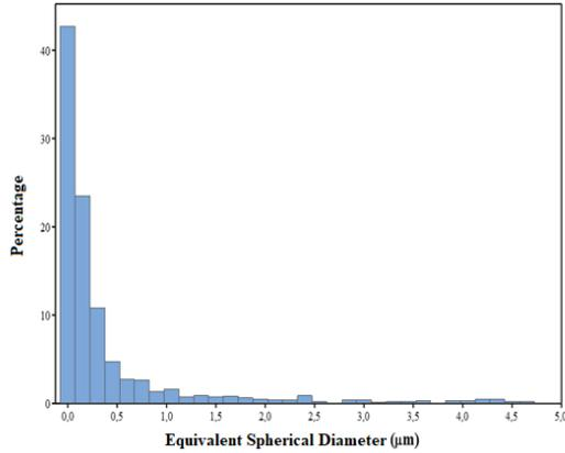
**Figure 12** - Pore distribution of the L35A65 membrane.
