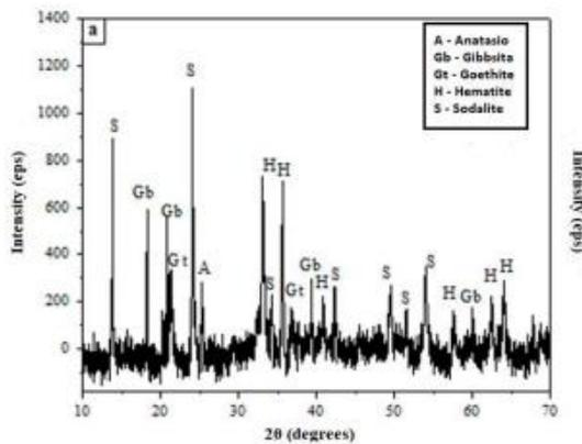
**Figure 5** - X-ray diffraction from the Red Mud.
