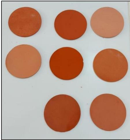
**Figure 7-** Different compositions of ceramics membranes after sintering.
