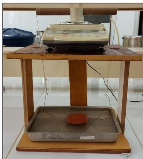
**Figure 3** – Apparatus used to determine the physical properties of membranes: Absorption in Water (WA), Apparent Density (AD) and Apparent Porosity (AP).
