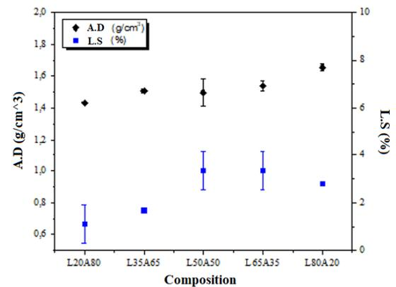
**Figure 11** - Physical properties of membranes: Apparent Density (g/cm<sup>3</sup>) and Linear Shrinkage (%).
