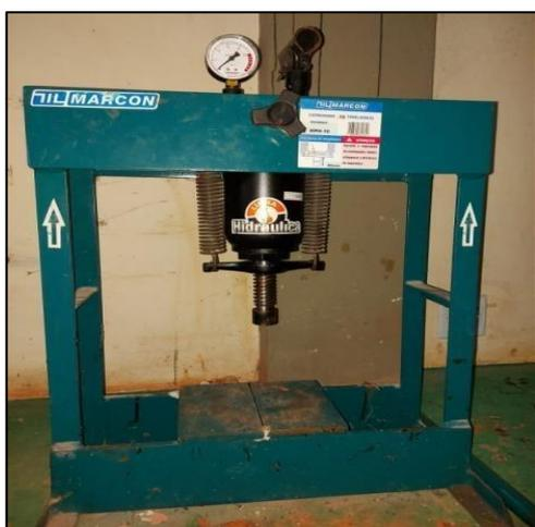
**Figure 2** – Hydraulic Press (MARCON-MPH-10).
