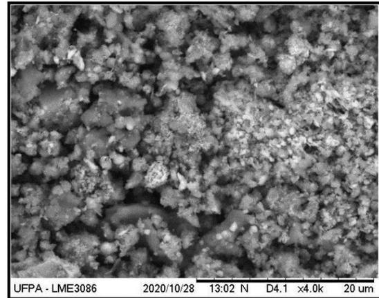
**Figure 8** - Electron Micrograph from the longitudinal section of L35A65 ceramic membrane with 4000x magnification.
