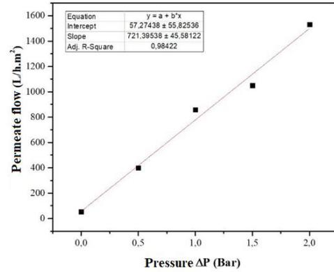
**Figure 13** - Hydraulic permeability of the L35A65 membrane.
