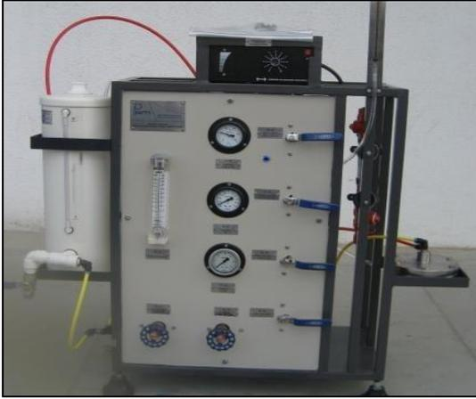
**Figure 4** - Microfiltration (MF) system used to test confectioned membranes.
