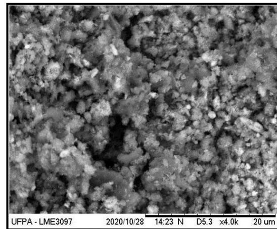
**Figure 9** - Electron micrograph of the transversal section of the L35A65 ceramic membrane at 4000x magnification.
