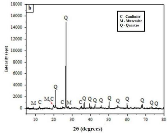
**Figure 6** - X-ray diffraction from the Clay.
