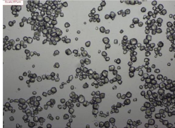
**Figure 18** - Microscopy of the unheated starch solution.
