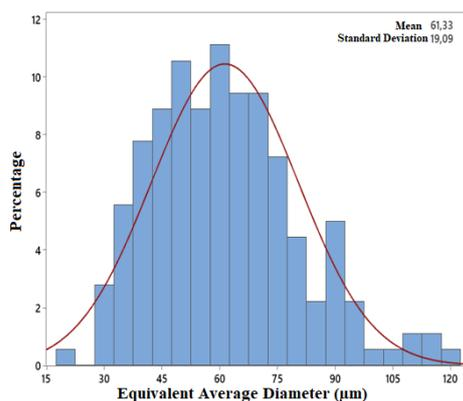
**Figure 21** - Count and distribution of the mean equivalent diameter of the starch solution after heating.
