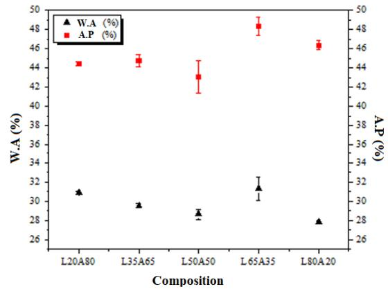
**Figure 10** - Physical properties of membranes: Water absorption (%) and Apparent Porosity (%).
