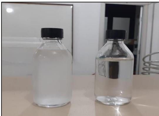
**Figure 15** - Samples of starch solution from concentrate (left) and permeate (right).
