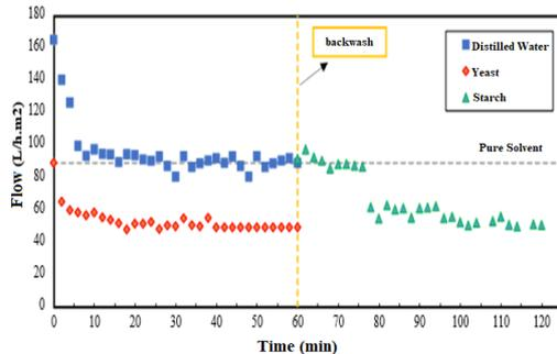
**Figure 14** - Permeate flow for distilled water, yeast, and starch solution.
