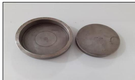
**Figure 1** – Mold prepared with VC 131 steel.
