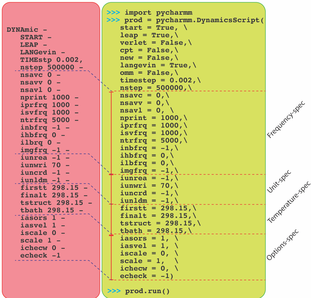
Figure 3: Configuring and performing a molecular dynamics run using the ‘DynamicsScript’ class in pyCHARMM. The correspondence with the DYNAMIC command in CHARMM in terms of the use of command keywords as function arguments to instantiate an object of the class is shown and the presence of different categories of run parameters is illustrated. In Figure S1 , the use of Python dictionaries for the same purpose is shown.
