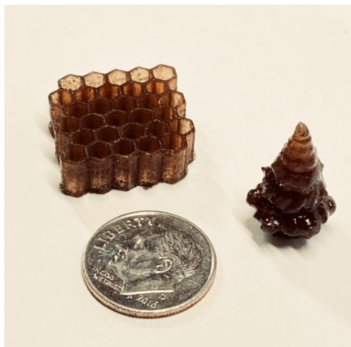
Figure 3. Examples of objects 3D printed using T2 75 H resin to demonstrate the print resolution and even dispersion of the LMA. A honeycomb and a tree are shown with a U.S. dime included as a reference.
