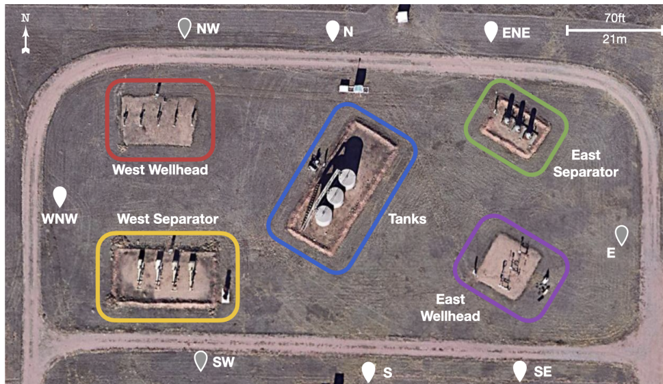
Figure 1: Satellite imagery of the Methane Emissions Technology Evaluation Center (METEC) facility. Source locations are marked with colored boxes. CEMS sensor locations are marked with pins and are named based on their geographical position. Pins with gray interiors indicate that the corresponding sensor measures wind speed and direction in addition to methane concentrations.
