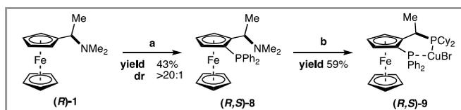
**Scheme 5.** Synthesis of (*R,S*)-Josiphos-copper Complex. Reagents and conditions: (a)  $n\text{BuLi}$  (1.2 equiv), chlorodiphenylphosphine (2 equiv),  $\text{Et}_2\text{O}$ ; (b) dicyclohexylphosphane (1.1 equiv), AcOH; then  $\text{CuBr DMS}$  (1.0 equiv), DCM (0.07 M).
