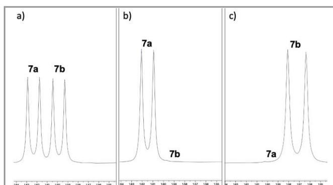
**Figure 1.**  $^1\text{H}$  NMR (600 MHz) spectroscopy signals of methyl protons (highlighted in blue) of compounds **7a** and **7b**; (a) mixture of both diastereomeric salts; (b) **7a** (>20:1 dr); (c) **7b** (>20:1 dr).
