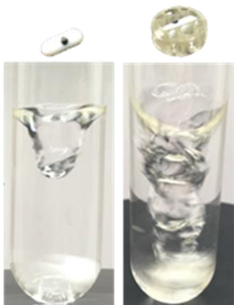
Figure 5: The vortexing ability of a conventional stirrer at 1400 rpm (left) versus that of its 3D printed congener (right).
