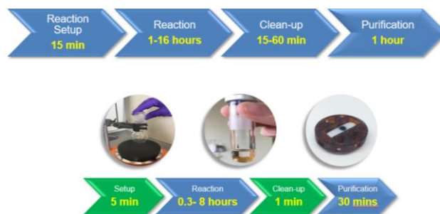
Figure 1: Illustration of standard chemical workflow (Top) versus our approach via the use of 3D printed catalyst embedded stirrer devices (Bottom).
