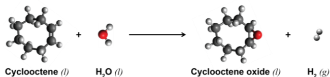
Scheme 1. Electrochemical cyclooctene epoxidation with water as the sole oxygen source.
