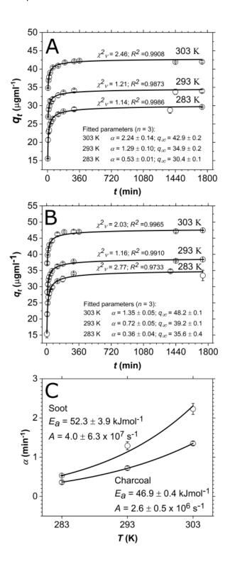
342 Figure 3. Kinetic experimental data (empty circle) with the Ritchie kinetic model (full line),
