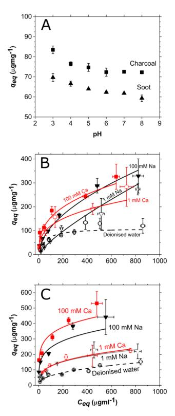
Figure 2. a) DNA adsorption capacity decreases as pH increases in solution with 100 mM NaCl and with initial DNA concentration of 50  $\mu gml^{-1}$ . Adsorption isotherms for b) soot and c) charcoal. Experimental data are represented with symbols and best fits with lines (Freundlich model except for soot in 1 mM CaCl<sub>2</sub> solution and deionised water that was best fit with the Sips model). All uncertainties given as standard deviation.
