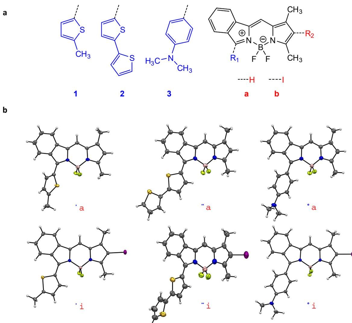
**Fig. 1:** a, Chemical structures of **1a** - **3a**, as well as **1b** - **3b**. b, Ellipsoidal representations of the X-ray crystal structures of **1a** - **3a**, and **1b** - **3b** (ellipsoids drawn at 50% probability). For clarity, only one out of two molecules in the asymmetric unit is shown for **1a**, the minor orientation of the disordered terminal thiophene unit has been omitted for **2a**, and one DCM co-solvent molecule has been omitted for clarity for **2b**.
