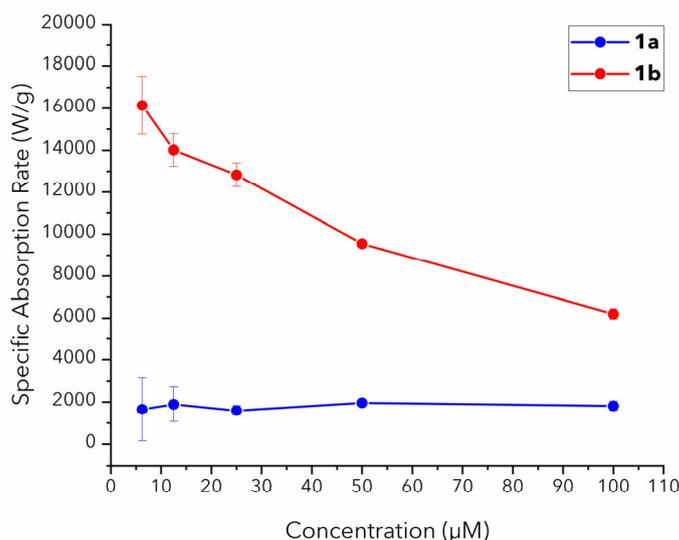
**Fig. 4:** Specific absorption rates (W/g) of **1a** and **1b** plotted versus the concentration. A clear increase of the SAR values for lower concentrations of **1b** is observed, while the SAR of **1a** virtually shows no concentration dependency.
