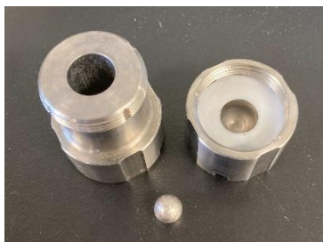
Figure S2. Stainless jars and balls used in this study.
