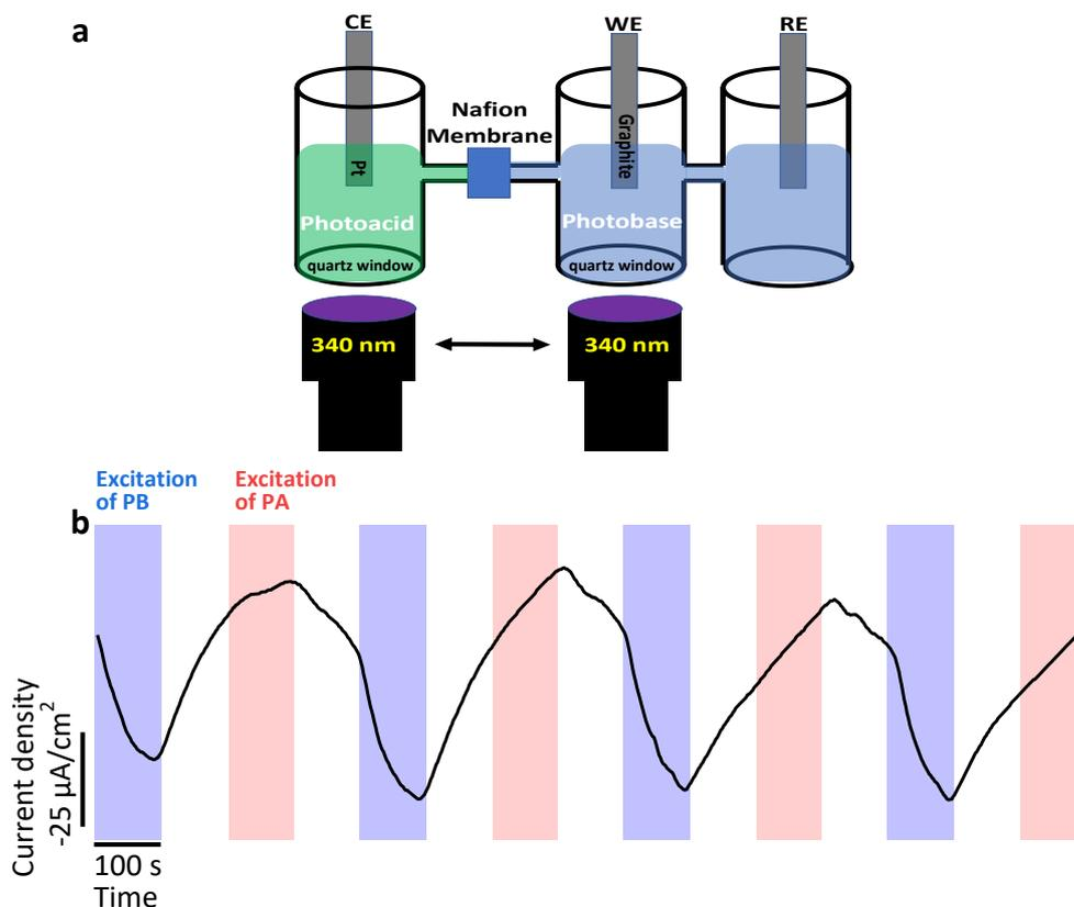
**Figure 7.** H-cell setup. Photocurrent control by alternate irradiation of 6AQ (PB) and 2N6S (PA). **a.** A schematic representation of the H-cell along with other components of the setup. **b.** Changes in current upon alternate irradiation of 6AQ and 2N6S at the bias of -1V.
